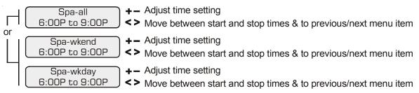
This menu is only available if the system has been setup for "pool and spa". During the programmed spa time, the Aqua Plus will turn on the filter pump and move the pool/spa valves into the "spa-only" position. The heater will automatically heat the spa up to the programmed spa temperature (page 7). This programmed spa operation will take precedence over all other automatic functions, only manual operation of the filter button or pool/spa valve button will override this function.
