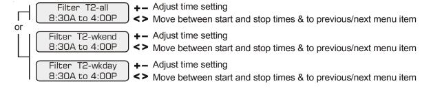
For one speed pumps, this is the second filter timeclock
