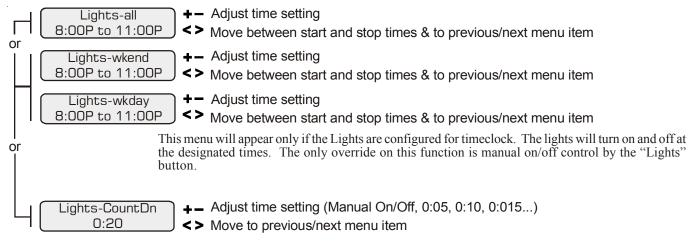
This menu will appear only if the Lights are configured for countdown timer. This setting is the time after you manually turn on the lights until the Aqua Plus automatically turns off the lights. You can also manually turn off the lights at an earlier time by pressing the LIGHTS button. If the Lights relay is on during the programmed off time, it may be because of freeze protection.
