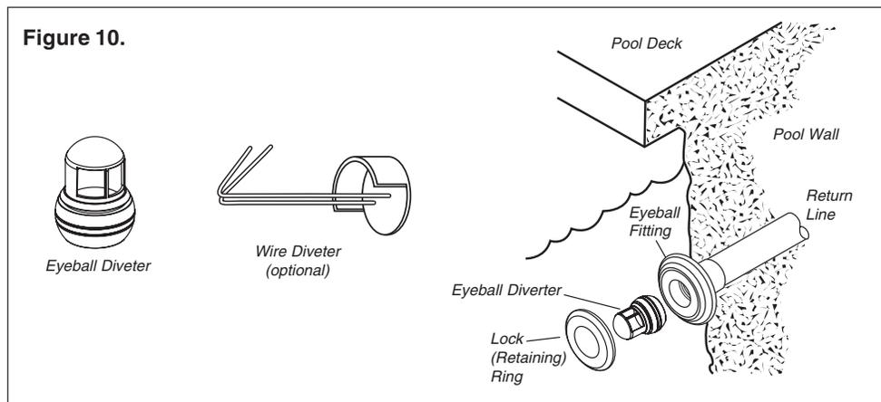
**IMPORTANT: The eyeball diverter must fit snugly into the eyeball fitting.** Some eyeball fittings, like Aqua Leader or Olympic, may be too large for the eyeball diverter. In this situation, use the outer ring supplied with your E-Z Vac® to adjust for the discrepancy in size.
