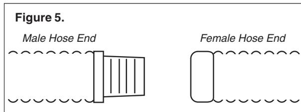
Begin by attaching the female end of a male/female hose section to the swivel head of your E-Z Vac<sup>®</sup>, see Figure 6. Connect two more male/female hose sections to the first section. Then install the hose weight near the male end of the third hose section as shown in Figure 6. Finally, assemble the complete hose, ending with the male/female section. To ease the assembly of the hose, dampen the hose ends with water as you assemble them together.
