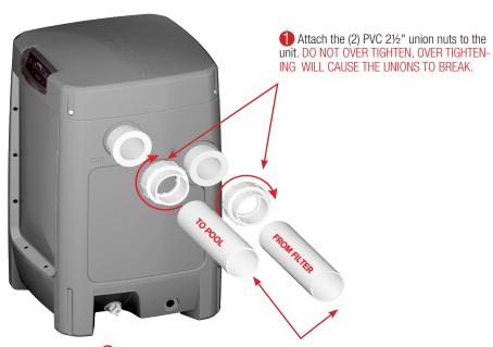
② After cutting pipes to length, debur all cut pipe to ensure shavings don't plug critical points internal to the unit. Use PVC solvent cement to glue pipes into the union sleeve. NOTE the inlet and outlet pipe positions.
