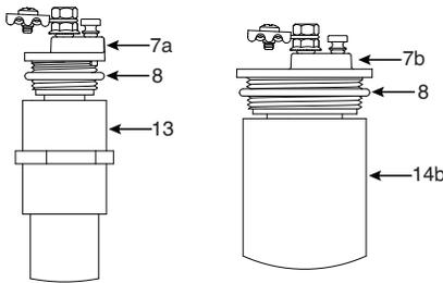
Apply O-ring lubricant (not supplied) to the large O-ring (8) on the TechNode Cap (7a or 7b). Thread the Anode Cap into the threaded end of the Female PVC Adapter (13) or the 2" Clear Anode Housing (14b) and tighten approximately 1/6 turn after the O-ring contacts the housing.
