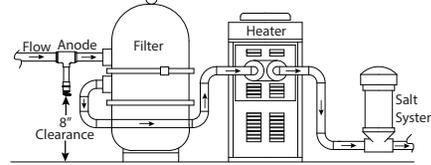
Decide where to install the In-Line anode in the pool plumbing. **For proper anode function, the anode must be installed up-stream of the pool heater and salt system generator. Clearance: Make sure to provide adequate clearance for removing the zinc from the plumbing.**
