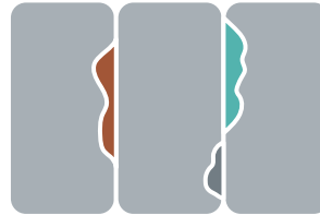
Galvanic corrosion occurs when different metals touch
